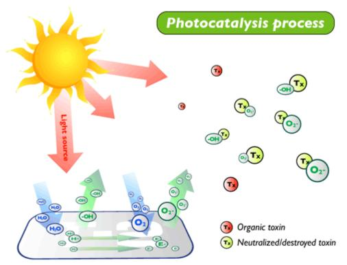
Using energy from light, T-2 creates two oxidation reactants: hydroxyl radicals and superoxide anion. These reactants decompose toxic organic substances through oxidation.
