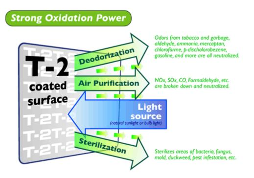
Hydroxyl radicals are among the most powerful oxidizing radicals, even stronger than chlorine, ozone, and peroxide. They act as very powerful disinfecting agents by oxidizing the cells of microorganisms, causing rupture of the cell and leakage of vital composition.
